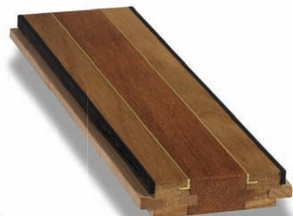
The profiles shown here consist of two or more parquet strips with one or more three-ten-mm thick strips of neoprene in between. The models are joined to the strips by decorative brass profiles. When the wood expands, the neoprene strips are compressed. This allows the profile to absorb a large amount of swelling and to use the stored energy to return the floor elements to their original positions when the swelling subsides.
