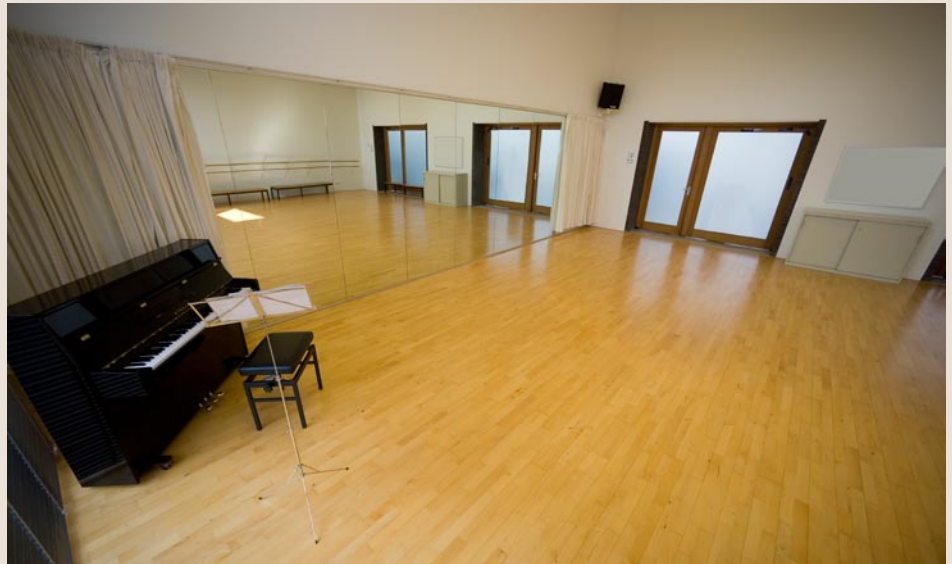
Below the solid beech parquet, a 7mm foam and a 3mm ‘Elastilon Strong’ mat guarantee uniform elasticity at every single spot on the floor.
